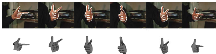
Fig. 6. Tracking a pointing hand in front of clutter. The images are shown with projected contours superimposed (top) and corresponding 3D avatar models (bottom), which are estimated using our tree-based algorithm. The hand is translating and rotating. A 2D deformable template would have problems coping with topological shape changes caused by self-occlusion.
